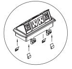
Use phillips head screwdriver to tighten locking cams snuglyto the work surface. To Access back screw, flip back power encloser past stops. After locking cam is secured, rotate power enclosure back into place. **Do not overtighten.**
